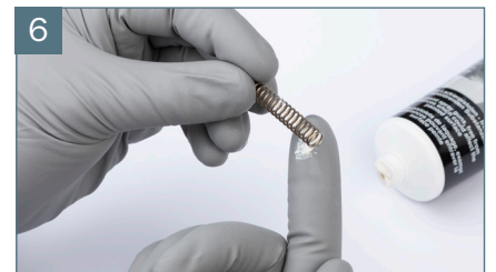
Grease and insert paint needle spring
