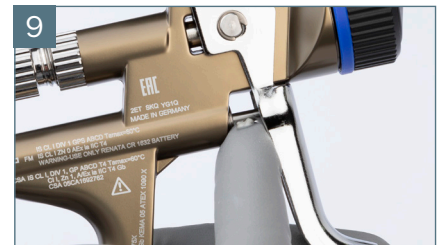
Grease visible part of air piston rod
