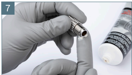
Grease thread of material flow control screw
