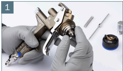
Assembly of the fluid tip
