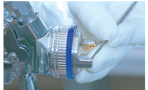
Manual adjustment: Each nozzle set is manually "tuned" in order to ensure an optimum spray pattern.
