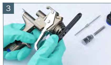
And finally, unscrew fluid tip with the ring spanner integrated in the universal spanner.
