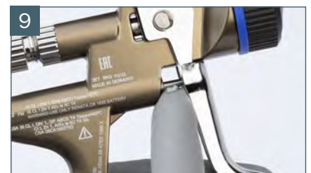
Grease visible part of air piston rod
